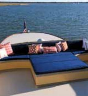
A comfortable settee on the upper deck was actually purpose-built to house the air handler for the main salon's air-conditioning system.
